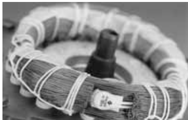
Fig. 50 Thermal switch incorporated in windings
