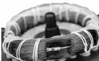
Fig. 48 PTC sensor incorporated in windings
