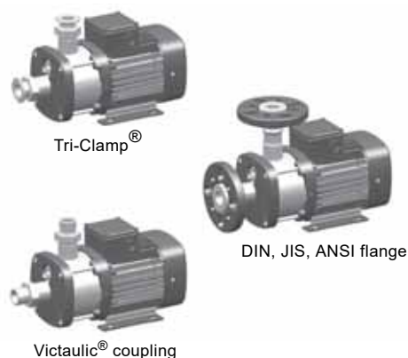
Fig. 37 Examples of pump connections
